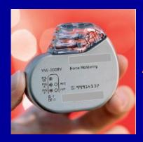
A highly reliable RF transmitter integrated into the ICDdevice sends patient and device data on command
